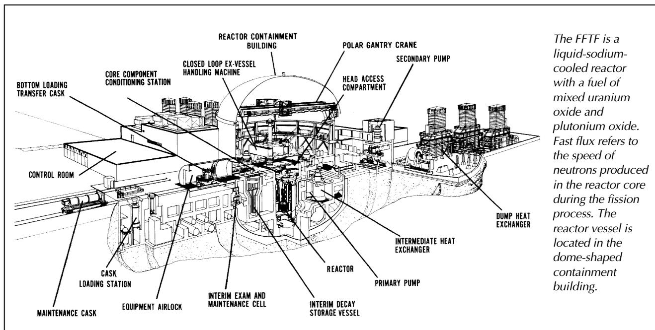
*The FFTF is a liquid-sodium-cooled reactor with a fuel of mixed uranium oxide and plutonium oxide. Fast flux refers to the speed of neutrons produced in the reactor core during the fission process. The reactor vessel is located in the dome-shaped containment building.*
