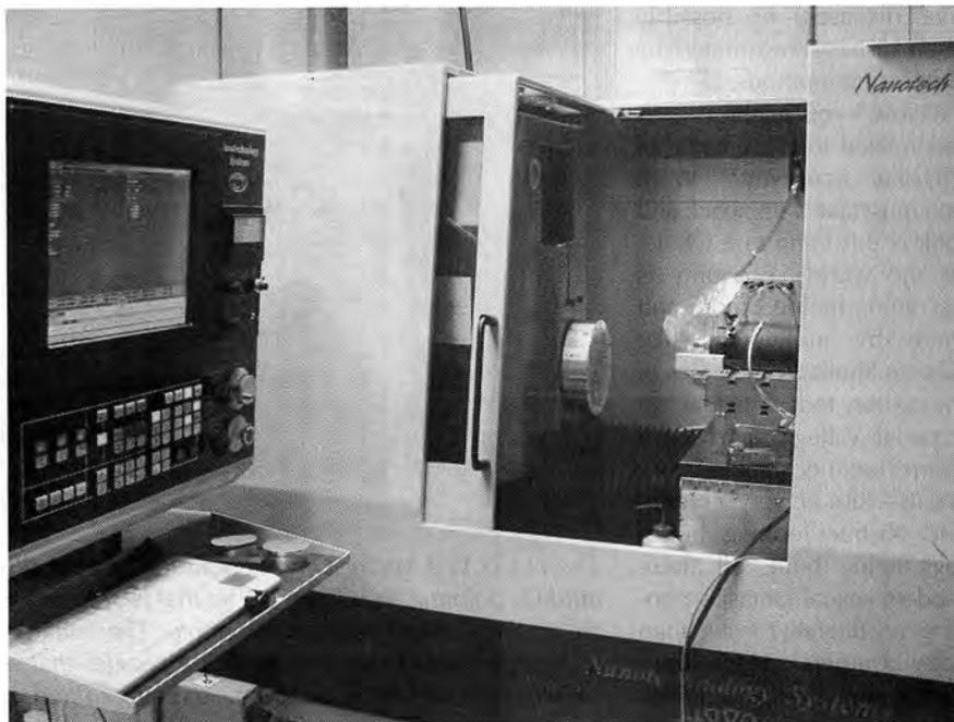
*Nanotechnology System's Nano-Lathe. It can shave metal to specifications as close as 1,000,000th of a millimeter.*
