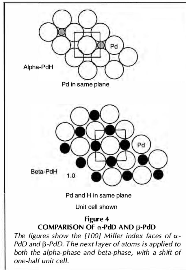
mined by comparing the expected lattice volume, based on the composition, to the measured volume.[114] In forming the  $\beta$ -phase, atoms of Pd shift to allow D atoms into equivalent positions, as shown in Figure 4. Hydrogen lies in the plane, forcing Pd atoms further apart, and occupying the so-called octahedral position. These positions can be filled or empty in a random manner up to a completely filled lattice at PdH<sub>1.0</sub>.
