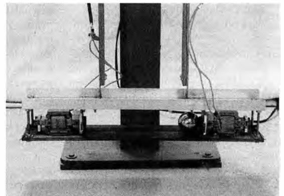
B The push-plates of the solenoids are magnetized.
