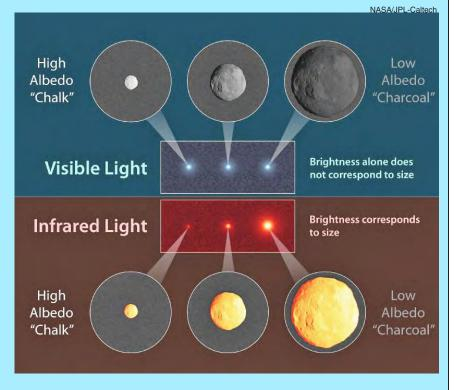
same three asteroids. Because infrared detectors sense the heat of an object, which is more directly related to its size, the larger rock appears brighter. In this case, the brightness of the object is not strongly affected by its albedo, or how bright or dark its surface is. When visible and infrared measurements are combined, the albedos of asteroids can be more accurately calculated.
