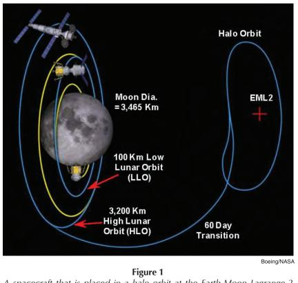
A spacecraft that is placed in a halo orbit at the Earth-Moon Lagrange-2 point (EM L2) would need very little energy to stay in place. This region in space is about 64,000 km farther from Earth than the Moon is, and would be a low-energy transfer point to lunar orbit, as seen here.
