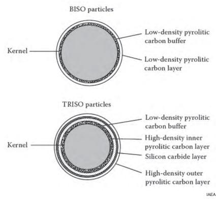
*Bi-isotropic ("biso") and tri-isotropic ("triso") nuclear fuel pellets. Both pellets contain a kernel of uranium fuel, coated by several layers of material.*
