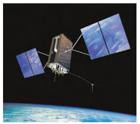
Research Center for Earth Operative Monitoring GPS satellites, whose signals may be used to measure ionospheric characteristics to aid in forecasting earthquakes.
