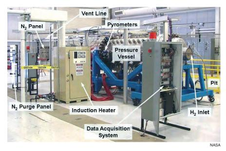
The Nuclear Thermal Rocket Element Environmental Simulator (NTREES), at NASA's Marshall Space Flight Center, is designed to closely approximate the conditions within a nuclear reactor, in order to test fuel element design for the NTR.
