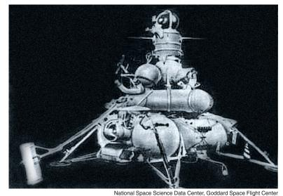
Luna 16 was the world's first robotic spacecraft to land on the Moon and return a sample of lunar soil to the Earth. That Soviet mission, in September 1970, followed the Apollo 11 and 12 U.S. manned missions. Luna 16 brought back, in an hermetically sealed container, 101 grams of material collected in the Sea of Fertility, on the Moon.
