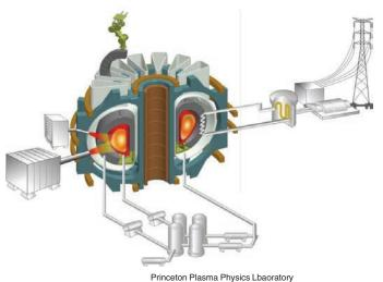
A schematic illustration of the K-DEMO fusion reactor.
