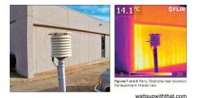
The heat island effect, which maintains an artificially higher temperature than surrounding areas, is visible in these infrared photos of two U.S. temperature stations.
