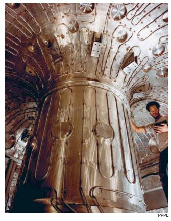
Inside a large tokamak. The tokamak geometry is more complex than an axisymmetric linear system, because of the shape of the magnet coils. Also, the interior parts are exposed to neutron fluxes. This is the PDX tokamak at Princeton, constructed in 1978.
