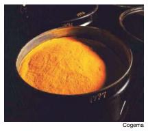
Uranium oxide (known as yellowcake), is the raw material processed into nuclear fuel. It is converted to a gas and then "enriched" through gaseous diffusion or centrifuge processing to concentrate the fissionable uranium isotope, U-235. The non-fissionable isotope, U-238, constitutes all but 0.7 percent of natural uranium. Reactor fuel generally requires about 3-5 percent of U-235.
