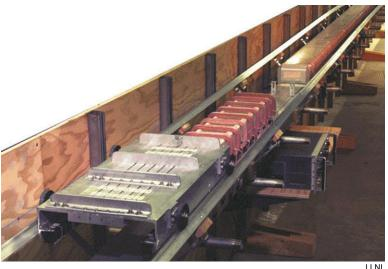
The 20-meter, scale-model test track used to test the Inductrack concept at LLNL. The test cart and electric drive circuit are in the foreground.
