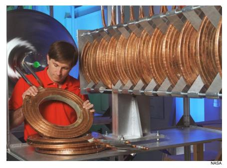
Fusion propulsion is crucial if man is to explore the Solar System, for it would shorten years-long journeys into manageable travel times. Here a NASA engineer inspects the solenoid magnets of a magnetic mirror-based fusion propulsion system under devel-
