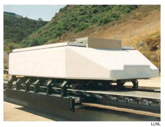
The General Atomics full-scale Inductrack test vehicle on the first section of its test track.
