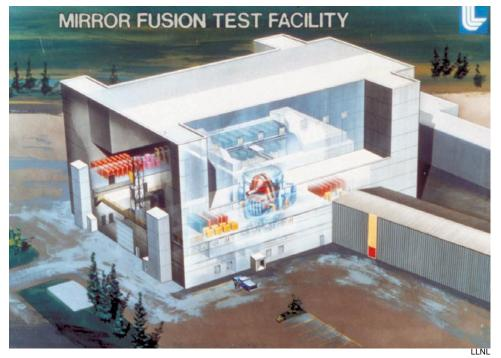
Artist's drawing of the Mirror Fusion Test Facility (MFTF), built at Lawrence Livermore National Laboratory in the 1980s. The vaccuum vessel at center is shielded in a seven-story-high concrete vault. The MFTF was forced to shut down soon after it was fully completed because of budget cuts. The U.S. magnetic fusion program was then narrowed to concentrate on tokamaks.
