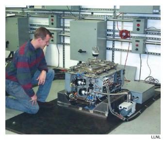
In this device, LLNL-designed Halbach-array generators are incorporated in AFS-Trinity Flywheel modules, producing 350kilowatts output from 25-centimeter diameter rotors.
