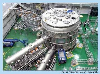
Korea's KSTAR fusion reactor at the National Fusion Research Institute in Daejeon, which reached its first plasma on July 15, 2008. It features fully superconductive magnets.
