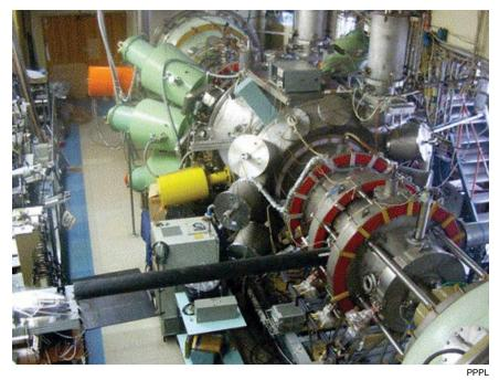
The Gas Dynamic Trap axisymmetric mirror machine at Novosibirsk, Russia, which has demonstrated plasma confinement with no turbulence.
