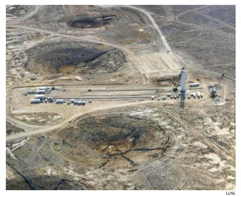
An aboveground diagnostic setup for an underground experiment at the Nevada Test Site. The data signals from a test explosion moved from the device, 300 meters underground via cables, up to the surface and along the surface to the instruments for reading the signals, housed in trailers on the site.
