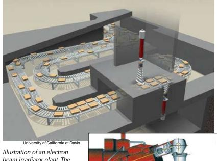
beam irradiator plant. The product moves on a conveyor belt and passes under a machine (inset) that generates and accelerates electrons, bending them to scan the product.
