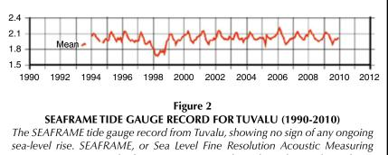
sea-level rise. SEAFRAME, or Sea Level Fine Resolution Acoustic Measuring Equipment, is a network of monitoring stations throughout the South Pacific region that provides data on sea level.
